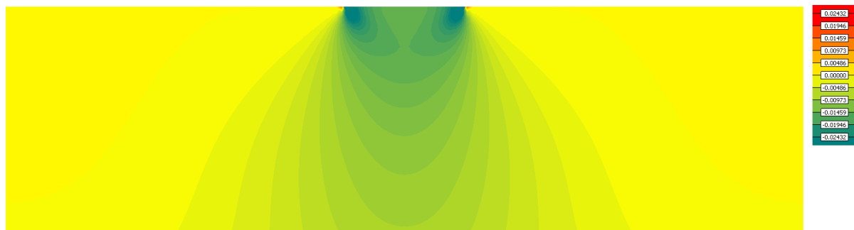
Figure 5.16 – Vertical stress distribution under the foundation [MPa]
